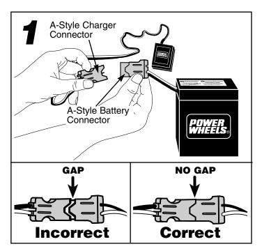
Plug the charger and battery connectors together.
